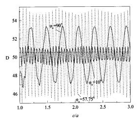
Fig. 5. Directivity of the same reflector near PEC earth as in Fig. 3 as a function of the normalized elevation, for in-zenith and near-grazing radiation.
