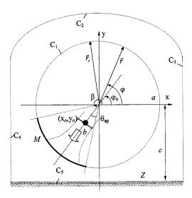
Fig. 1. Two-dimensional reflector antenna over impedance earth.
