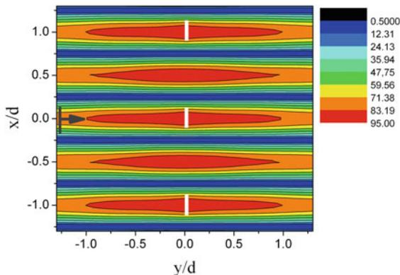
**Fig. 4.6** The near-field pattern on three spatial periods for the scattering of the H-wave by infinite grating of thin silver nanostrips (shown using *white boxes*) in the combined LSP-G resonance ( $\lambda = 643.116$  nm). Other parameters are the same as for Fig. 4.5
