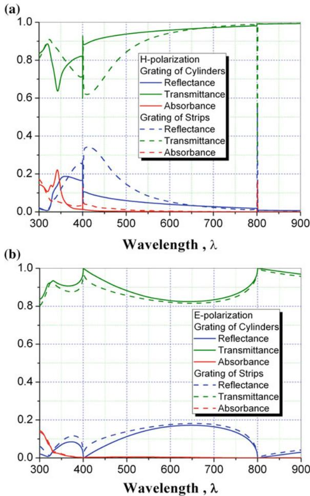
**Fig. 4.8** Optical characteristics spectra of infinite silver gratings with period  $d = 800$  nm illuminated by the H-polarized (a) and E-polarized (b) normally incident plane waves. The strip width is  $2w = 150$  nm and the thickness is  $h = 50$  nm, while the wire radius is  $a = 48.85$  nm
