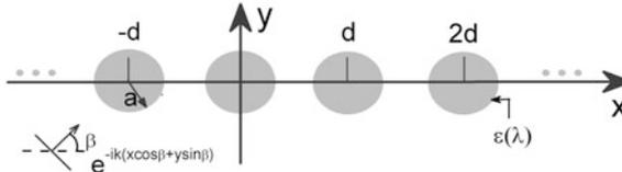
**Fig. 4.1** Cross-sectional geometry of an infinite grating made of circular cylinders or wires
