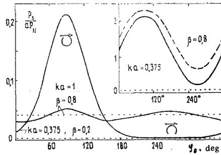
Fig. 4. Radiation energy as a function of the orientation of the coupling slot for  $\theta = 5^\circ$ . The dashed line corresponds to calculation using formula (13).
