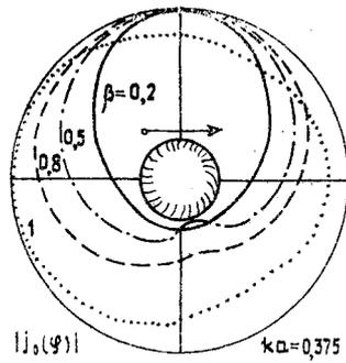
Fig. 2. Current distribution at the surface of the circular cylinder.
