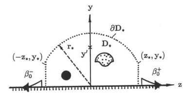
Figure 1. Two-dimensional geometry of localized scatterers near an impedance plane.
