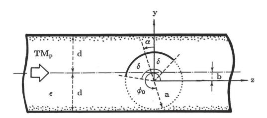
Figure 5. A particular 2-D geometry for a circular screen inside a dielectric slab. One of the natural guided modes is incident.
