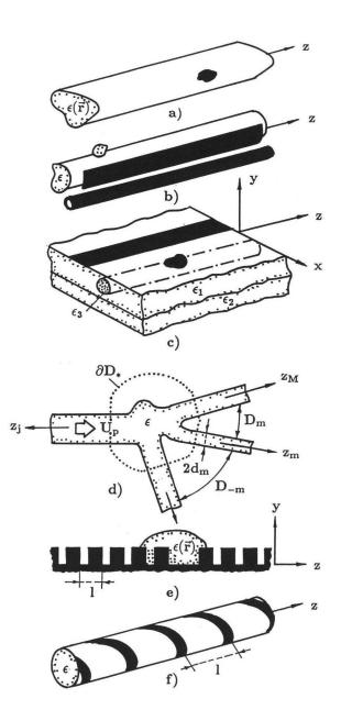
Figure 7. Examples of more complicated open waveguides containing localized inhomogeneities
