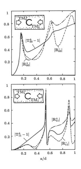
Figure 6. Amplitudes of the scattered field coefficients for a cavity shaped screen inside the two-mode slab. Incident mode is travelling either in the positive or negative z-direction.  $kd = 2.3, \epsilon = 2.25, b = 0, \theta = 30^{\circ}, \phi_0 = 0.$
