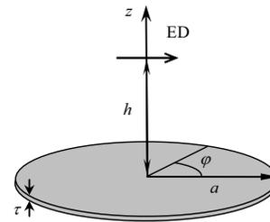
**FIGURE 1.** Geometry of a dipole above a dielectric microdisk.
