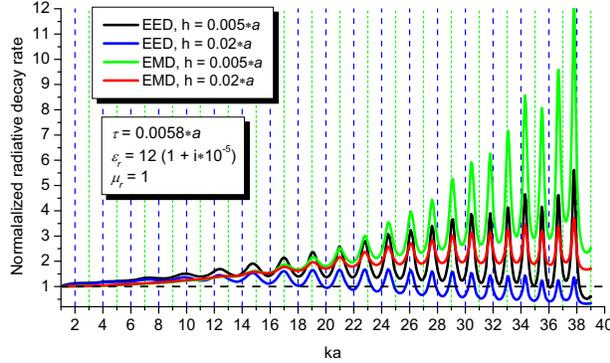
**FIGURE 3.** Normalized radiative decay rate vs. the dimensionless frequency parameter,  $ka$ .
