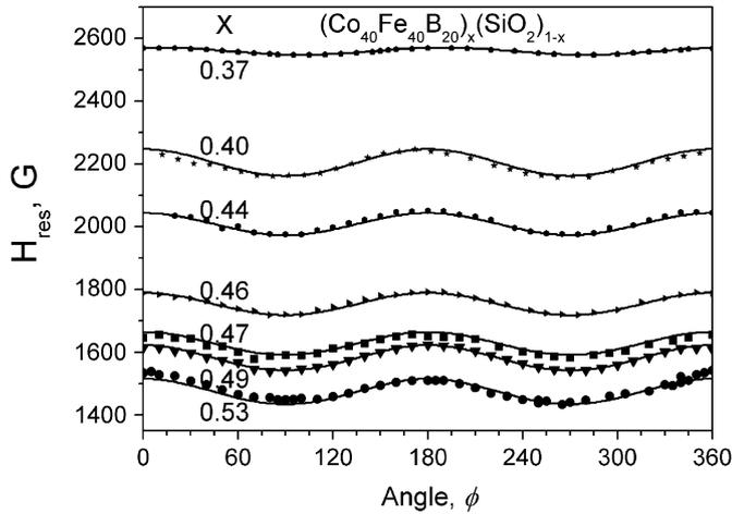
Fig. 2. Resonance field of the FMR spectra for the in-plane geometry. Solid lines are theoretical fitted curves, dots are experimental results.
