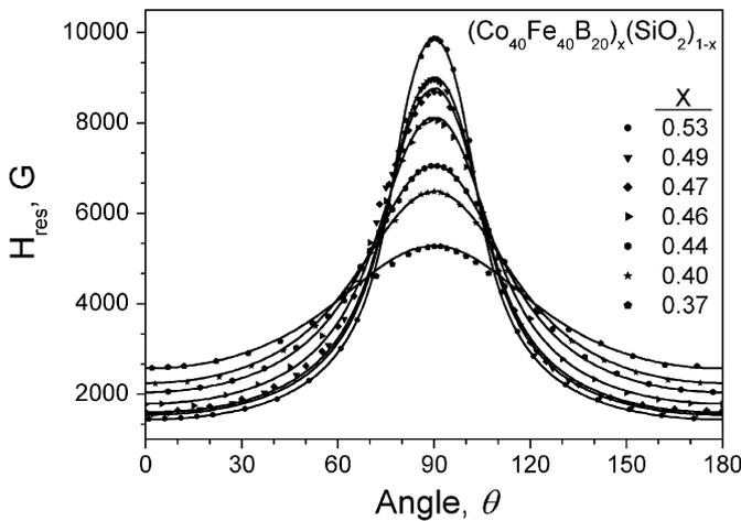
Fig. 3. Resonance field of the FMR spectra for the out-of-plane geometry. Solid lines are theoretical-fitted curves, dots are experimental results.
