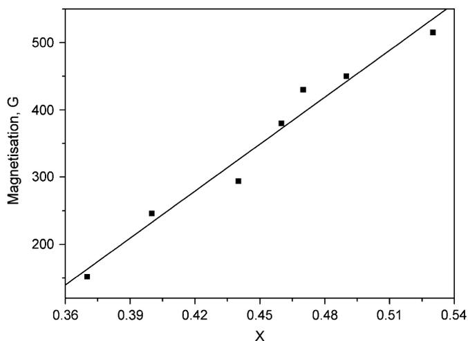
Fig. 4. Magnetization of the samples with respect to the concentration ( $x$ ).
