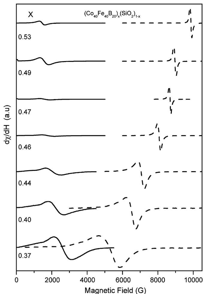
Fig. 1. FMR spectra of the  $(\text{Co}_{40}\text{Fe}_{40}\text{B}_{20})_x(\text{SiO}_2)_{1-x}$  granular thin films. Solid lines belong to the IPG cases, dashed lines belong to the OPG cases.
