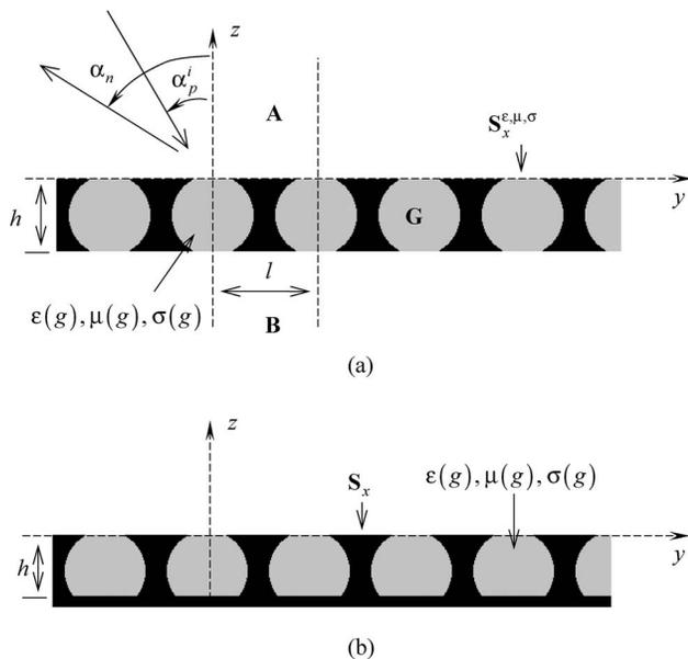
Fig. 1. Geometry of model problems: (a) semi-transparent and (b) reflecting plane gratings. All structures are homogeneous along the  $x$  axis.
