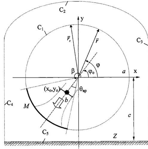
Fig. 1. Two-dimensional reflector antenna over impedance earth.
