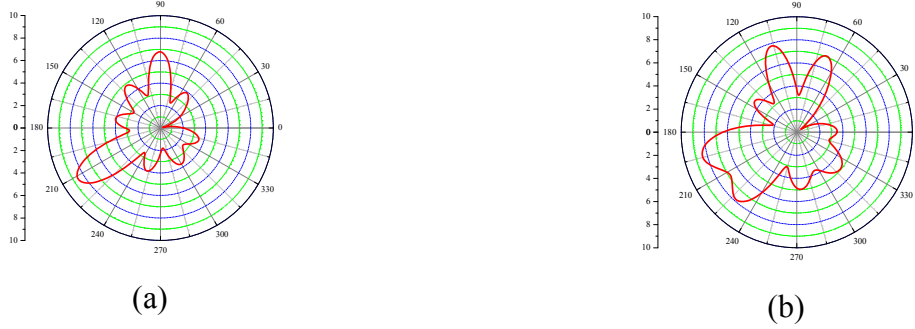
Fig. 10. Far-field patterns |H_z| of the whispering gallery modes in a spiral resonator: H_{7,1}^l (a) ka = 3.2962 , \gamma = 2.52 \cdot 10^{-2} ; H_{7,1}^h (b) ka = 3.2714 , \gamma = 3.048 \cdot 10^{-2} , N = 400 , spiral step height \delta = 1 , \beta = \pi/100 , \alpha_l = 2.63 .
