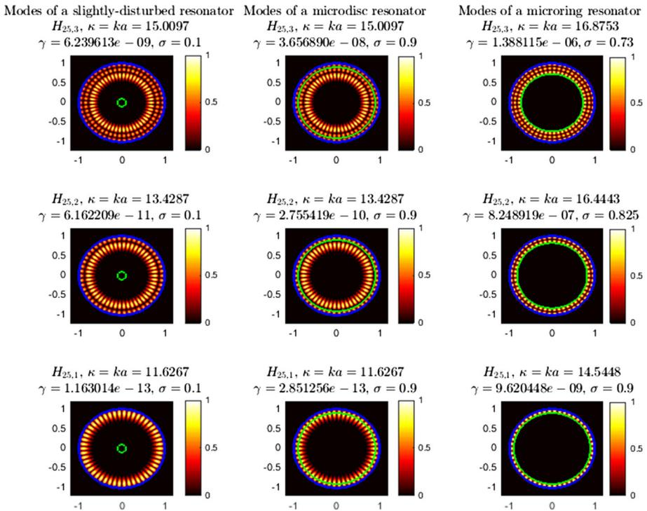
**Fig. 5** Near fields of the  $H_{25,n}$  modes for  $n = 1, 2, 3$  of slightly-disturbed microresonators (left column), microdisk resonators with the ring active region having  $\sigma = 0.9$  (central column), and microring resonators with some values of  $\sigma$  corresponding to stable calculations (right column)
