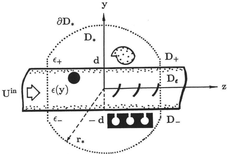
Figure 3. Two-dimensional geometry for a dielectric slab open-waveguide scattering.
