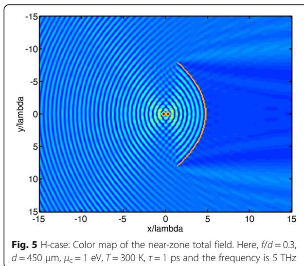
(this is  $7.5\lambda$ ). Note the splitting of the focal domain to two bright spots along the axis of symmetry – this is a side effect, at the given frequency, of the finite size of reflector. Besides, one can see clearly observable interference of the waves scattered by the edges of the parabolic reflector in front of it and the presence of shadow behind it. Still this shadow is not very dark because the graphene reflector is partially transparent.
