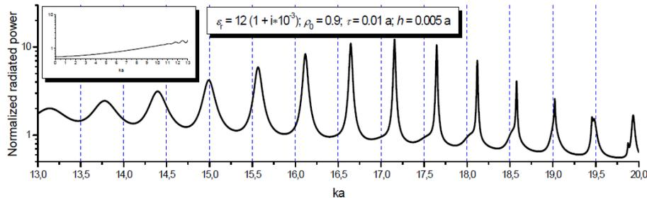
Fig. 2. Normalized radiated power for off-axis EED in the disk presence versus frequency  $ka$ .
