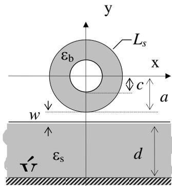
Fig. 1. WG-mode dielectric filter in a dielectric slab waveguide
