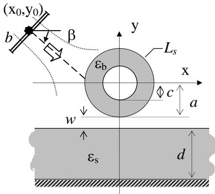
Fig. 5. WG-mode directional coupler in a dielectric slab waveguide
