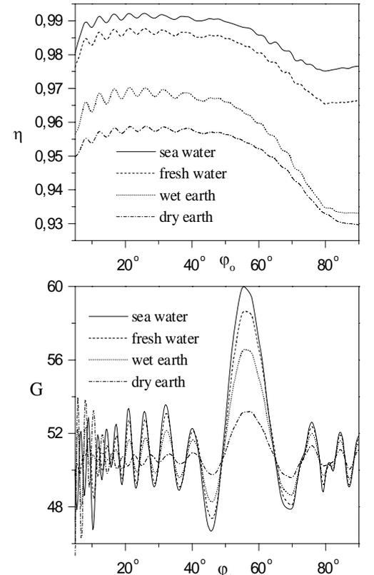
Fig. 10. Radiation efficiency  $\eta$  (a) and the gain of antenna  $G$  (b) for various types of the earth surface ( $c/a=1.01$ ).
