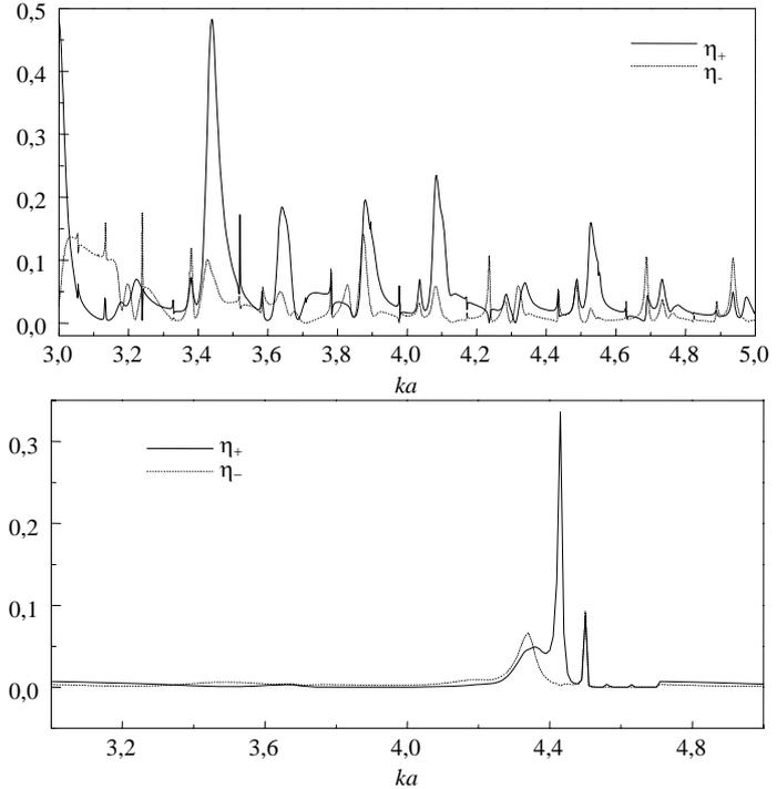
Fig.6. Right (left) moving guided wave coupling efficiencies ( $\eta_{\pm}$ ), H-polarization.  $kb=0.5$ ,  $y_0/a=1$ ,  $x_0/a=1$ ,  $\epsilon_b=50$ ,  $\epsilon_s=2.25$ ,  $\beta=180^\circ$ ,  $w/a=0.01$ ,  $d/a=0.6$ ; a)  $c/a=0$ , b)  $c/a=0.7$
