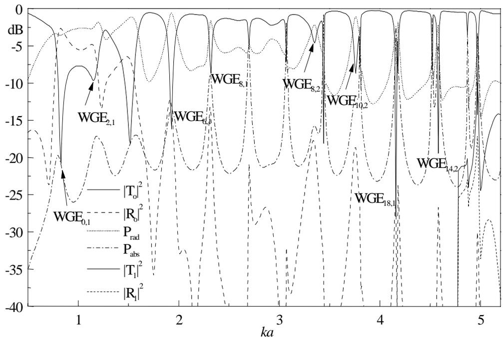
Fig. 2. Far-field scattering characteristics versus  $ka$  for the scattering from a circular cylindrical DR. ( $\epsilon_b=10+0.01i$ ,  $w/a=0.01$ ,  $d/a=0.6$ ,  $\epsilon_s=2.25$ ,  $w=b-a$ )
