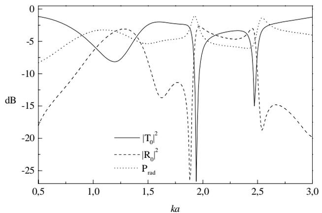
Fig. 8. Far-field characteristics for the scattering from a slitted cavity resonator:
