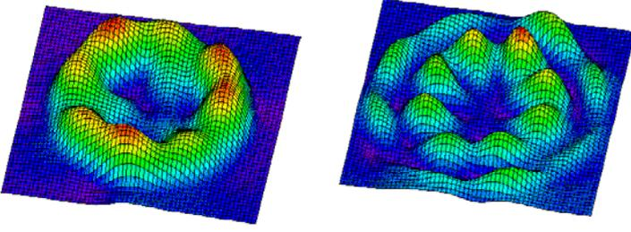
Fig. 3. The H-field spatial portraits at the resonances WGE<sub>6,1</sub> (left) and WGE<sub>8,2</sub> (right)
