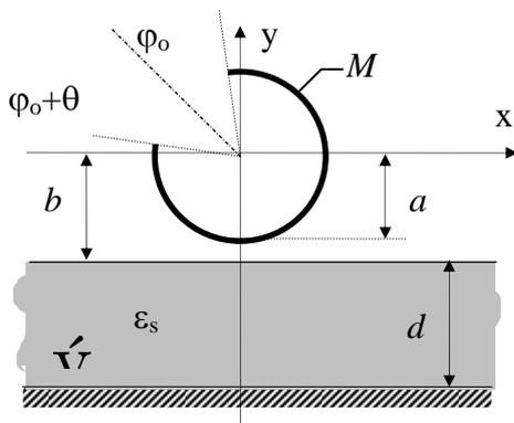
Fig. 7. Slitted cavity rejection filter in a dielectric slab waveguide
