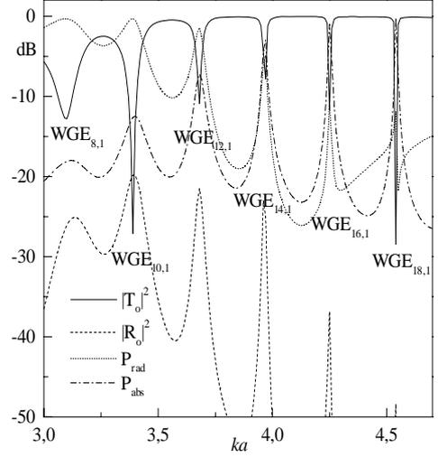
Fig. 4. Filter characteristics versus  $ka$  for the tubular dielectric resonator.
