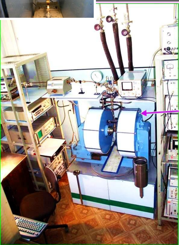
Experimental sample in resonator between the magnet tips
