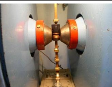
Experimental sample in resonator between the magnet tips
