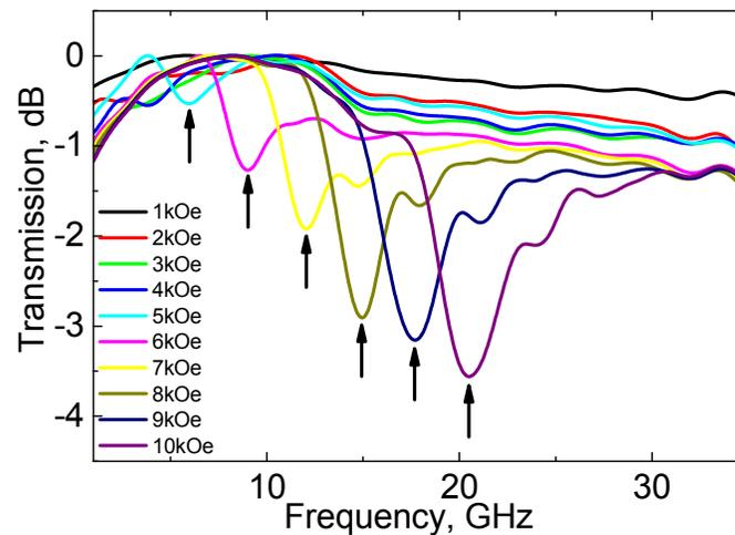
**FIG. 4:** Changes in the position of the magnetic resonance absorption peak on the frequency axis for ferrite specimen number 3 observed with the use of a microstrip transmission line with no width modulation
