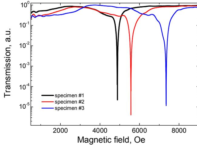
**FIG. 5:** Signals of the ferromagnetic resonance absorption observed in the test ferrite specimens at  $f_{TR} = 9.2$  GHz with the use of a resonance cell of the ferromagnetic resonance spectrometer on the basis of a planar photonic crystal with a “wire” medium
