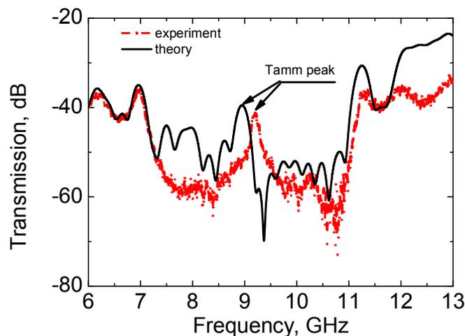
**FIG. 2:** Calculated and measured transmission factor spectra of the planar photonic crystal with a “wire” medium
