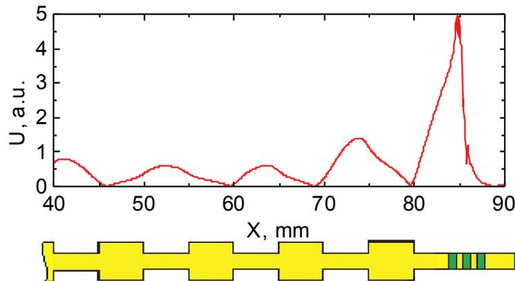
**FIG. 3:** Distribution of the high-frequency magnetic field in the planar photonic crystal contacting a “wire” medium
