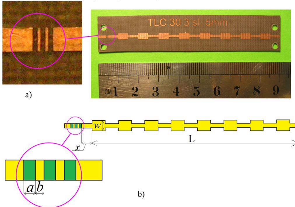
**FIG. 1:** Photo (a) and schematic representation (b) of the planar photonic crystal with a wire medium:  $L = 80$  mm,  $w = 3$  mm,  $x = 5$  mm,  $a = 2.5$  mm,  $a = 2.5$  mm, and  $b = 1.5$  mm
