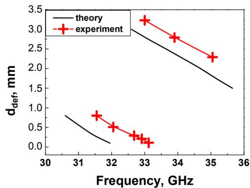
FIG. 5: Theoretical and experimental dependences of DM peak frequencies versus the defect layer thickness
