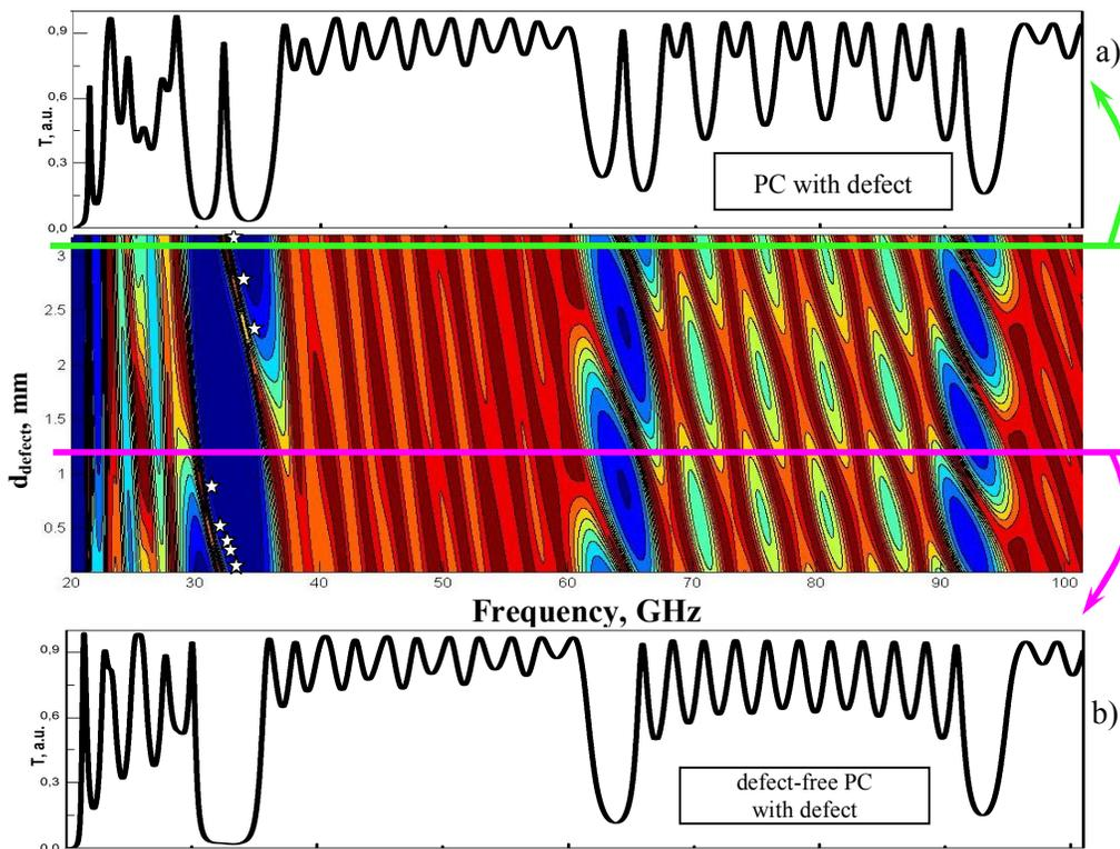
**FIG. 3:** (color online). Numerically calculated and experimentally measured (asterisks) the PC transmission spectra as a function of the defect layer thickness: a) the PC with defect; b) the “defect-free” PC
