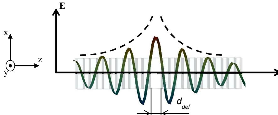
FIG. 4: Spatial distribution of the  $E$ -component of the microwave field at the DM frequency
