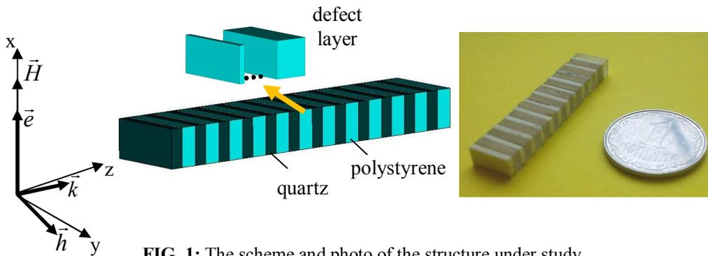
FIG. 1: The scheme and photo of the structure under study
