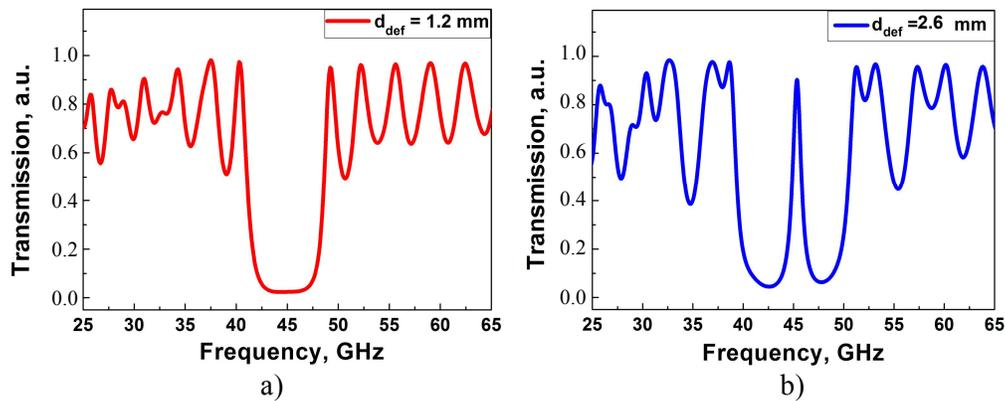
FIG. 2: The typical transmission spectra of the PC being studied: a) defect-free PC ( $d_{def} = d_p = 1.2$  mm); b) PC with defect ( $d_{def} = 2.6$  mm)
