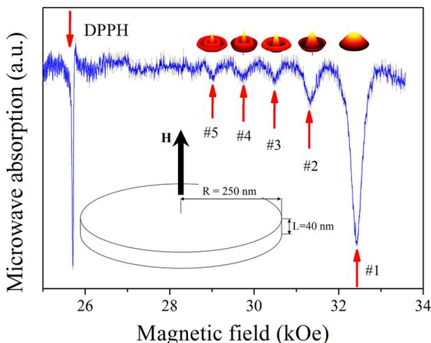
FIG. 1. Experimental spectra of array of circular Permalloy dots at 72.5 GHz. The inset shows disc dimensions and orientation of external magnetic field. Profiles of zero-order Bessel functions are shown above corresponding resonance peaks.
