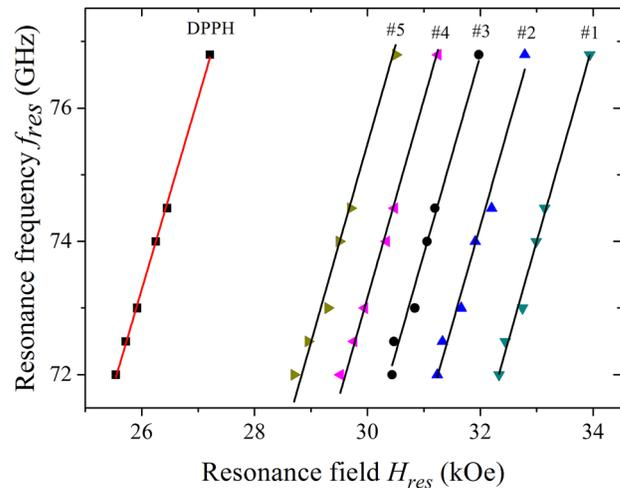
FIG. 2. Dependences  $f_{res}(H_{res})$  for different standing spin-wave modes at millimeter waves. Black lines are fits using analytical theory<sup>13</sup> with  $\gamma/2\pi = 2.96$  MHz/Oe and  $M_s = 795$  G.
