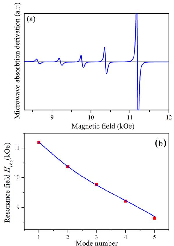
FIG. 3. (a) Experimental spectra of array of circular Permalloy dots at 9.86 GHz. (b) Dependence of the resonance field on the mode number. Points are experimental data, line is a fit using analytical theory<sup>13</sup> with  $\gamma/2\pi = 2.965$  MHz/Oe and  $M_s = 765$  G.
