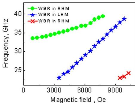
Fig. 8. (Color online) Frequency dependence of experimental resonance peaks position on magnetic field. One can watch as well an appearance of low-frequency mode (satellite one) of Wolf-Bragg resonance (WBR) in RHM at  $H > 9000$  Oe (red crosses).
