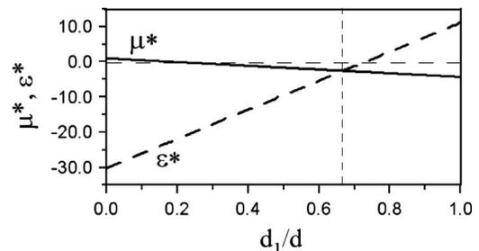
Fig. 4. The effective permeability and permittivity as a function of the thickness ratio.
