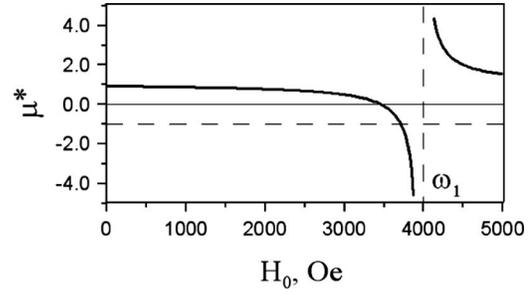
Fig. 3. The effective permeability as a function of external magnetic field.
