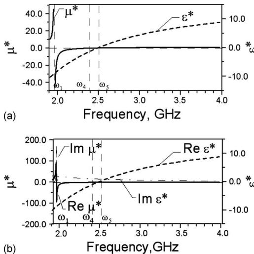
Fig. 2. The frequency dependencies of the effective parameters.
