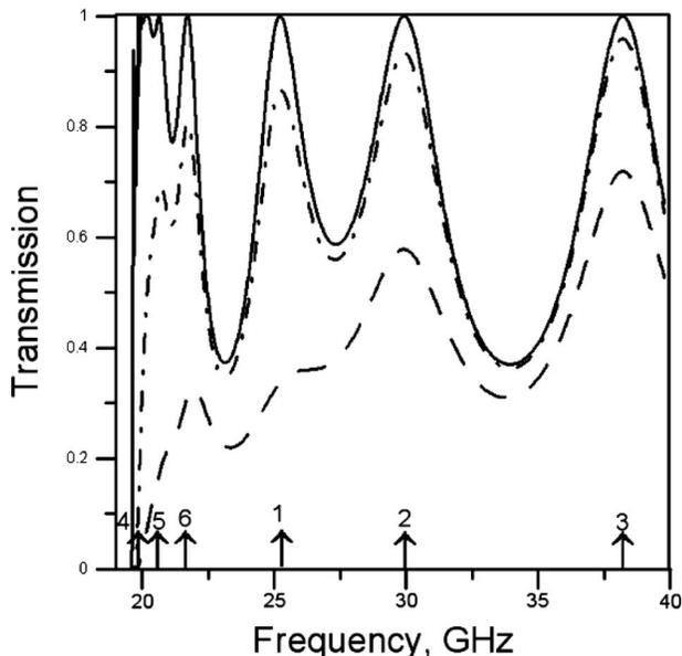
Fig. 5.  $|T|^2$  as a function of the frequency  $f$  for various collision frequencies.
