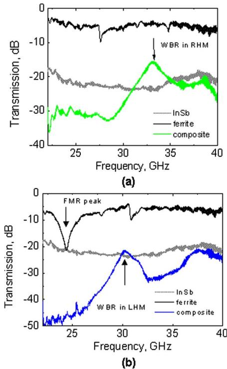
Fig. 7. (Color online) Transmission spectra of various structures: (a)  $H_0=0$  Oe: Wolf-Bragg resonance (WBR) in RHM; (b)  $H_0=6570$  Oe: WBR in LHM (1—ferrite layer; 2—InSb layer; 3—ferrite/semiconductor composite).
