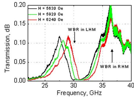
Fig. 9. (Color online) Transmission spectra of ferrite/semiconductor composite structure at various fields.
