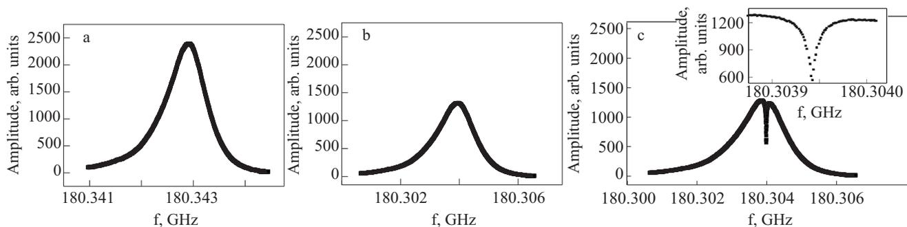
FIG. 2. Evolution of the resonance whispering gallery mode  $m=128$ . The resonator is in helium vapor at  $T=1.4$ – $1.6$  K (a); the resonator is immersed in He II at  $T=1.6$  K (b); the resonator is immersed in He II at  $T \approx 1.4$  K (c). The inset shows the narrow resonance absorption line on an expanded scale.
