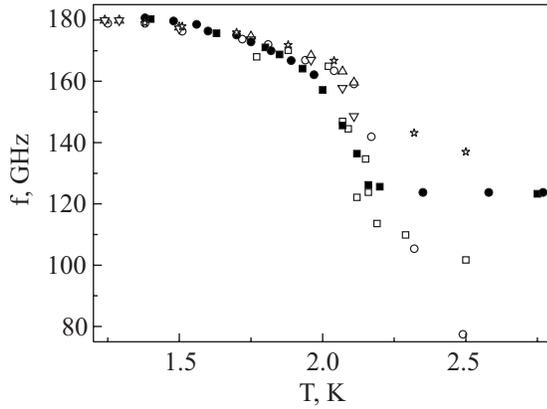
FIG. 5. Temperature dependence of the roton frequency obtained from the microwave measurements (present study (●), data of Ref. 1 (■)) and from neutron measurements (data of Ref. 4 (□); data of Ref. 5 (○); data of Ref. 6 (△, ▽); data of Ref. 7 (☆)).
