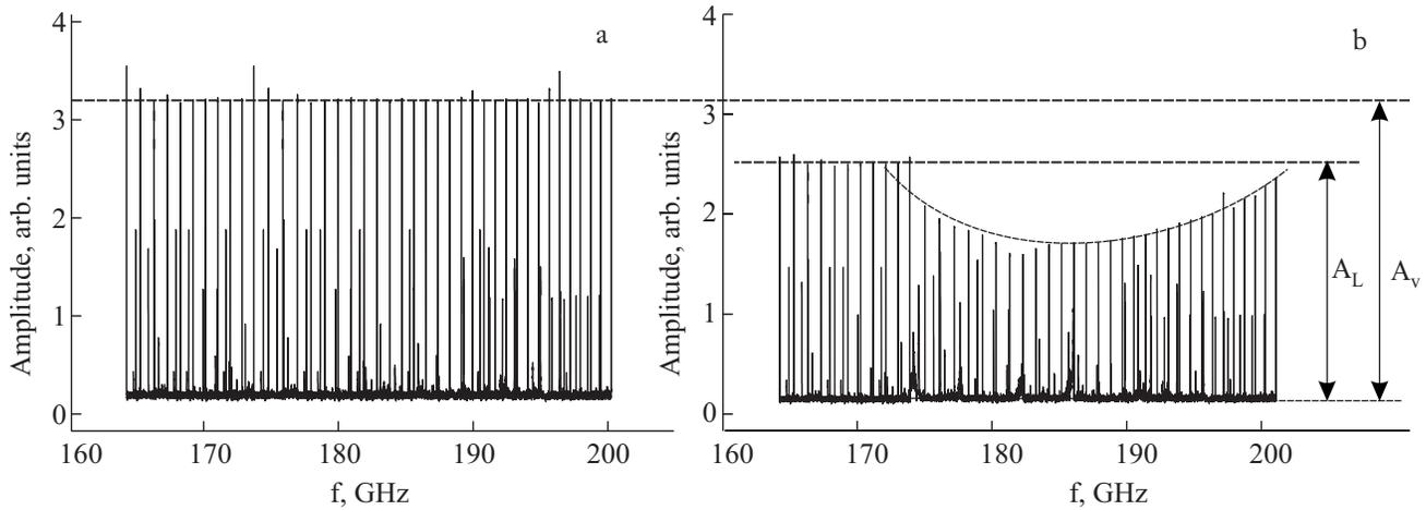
FIG. 1. Amplitude-frequency characteristic of the system at a temperature of 1.4 K: the resonator is found in the saturated vapor (a) or immersed in liquid helium (b). The upper dashed curve corresponds to the amplitude of the modes in the case of the vapor, while the lower dashed line is the boundary of the assumed dielectric loss in the liquid.
