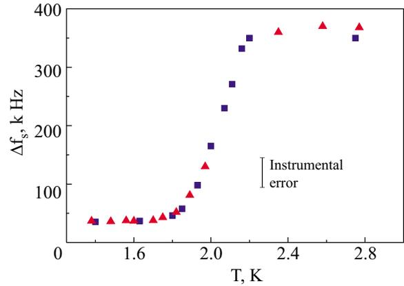
FIG. 4. Temperature dependence of the width of the narrow resonant absorption line: (■)—quartz resonator data, (▲)—leucosapphire resonator. Below a temperature  $T < 1.8$  K the data are limited by the resolving power of the spectrometer.
