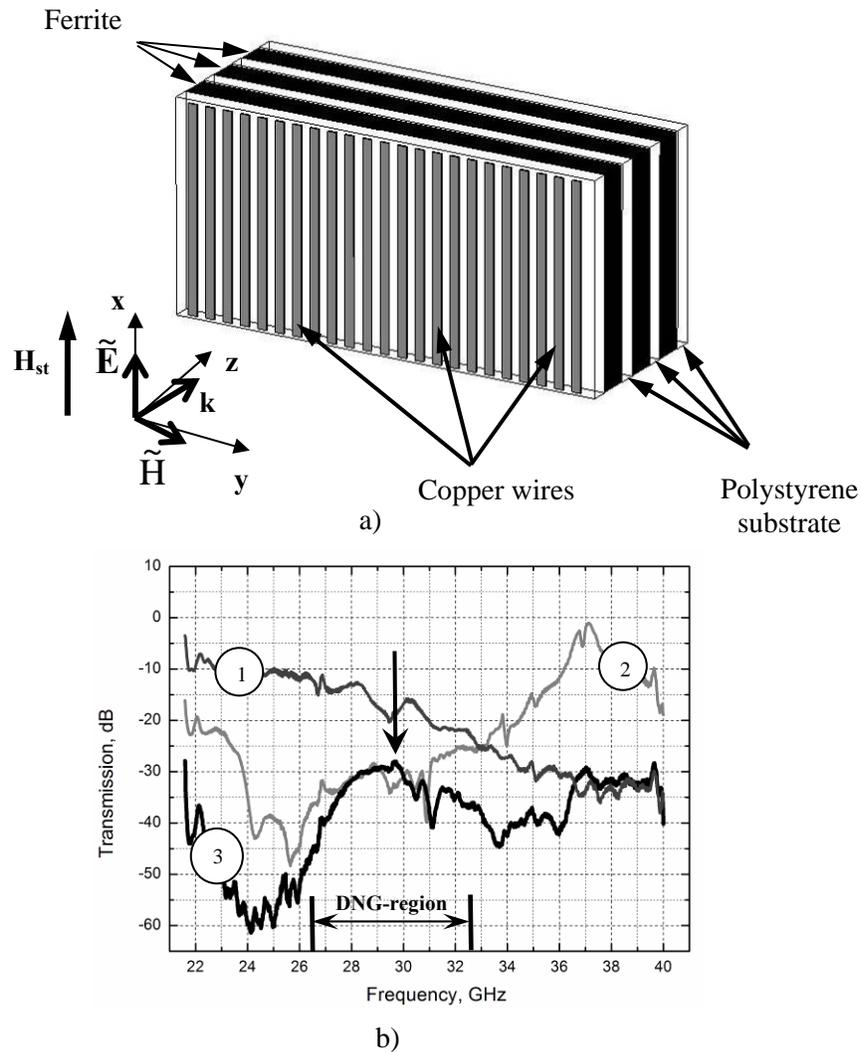
**FIGURE 1.** (a) Ferrite/wiremedium structure. (b) Experimental transmission coefficient for ferrite/wire-medium structure and its components.  $H_{st}=6.84$  kOe. (1)-WM: consists of 4 wire-media layers, (2) - ferrite- layer medium: consists of 4 ferrite layers, (3) – ferrite/wire medium structure: consists of alternated 4 wire-media layers and 3 ferrite layers.
