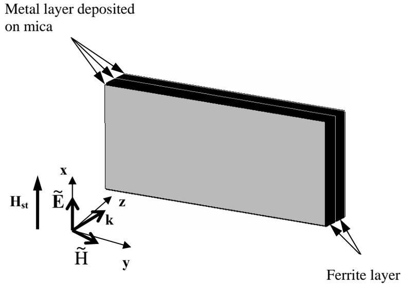
FIGURE 2. Ferrite/thin-metal-layer structure.
