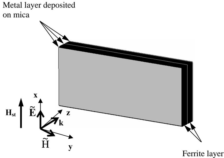
FIGURE 2. Ferrite/thin-metal-layer structure.
