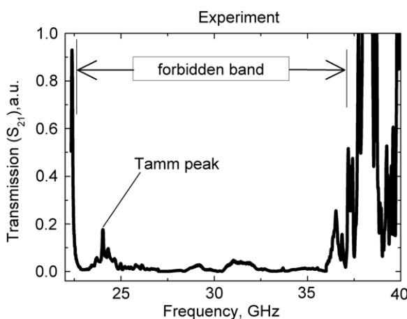
**Figure 4.** Experimental spectrum demonstrating the formation of the Tamm peak in the forbidden zone of the MPC for  $H_0 = 1880$  Oe.
