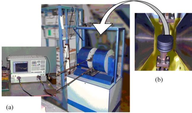
**Figure 1.** Photo of the test bench (a) and a typical MPC-structure between the poles of the magnet (b).
