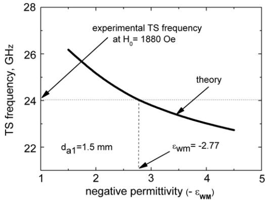
**Figure 5.** Variation of the TS frequency with the change in the WM permittivity  $\epsilon_{WM}$  for the magnetic field  $H_0 = 1880$  Oe at  $d_{a1} = 1.5$  mm.
