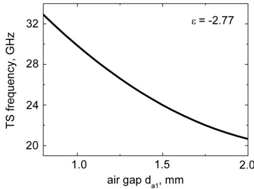
**Figure 3.** Dependence of the Tamm peak position on the value of the air layer thickness  $d_{a1}$ .
