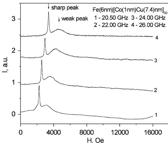
Fig. 1. Typical FMR absorption lineshape for Fe-buffered MLs  $\text{Fe}(6 \text{ nm})[\text{Co}(1 \text{ nm})/\text{Cu}(7.4 \text{ nm})]_{30}$ .
