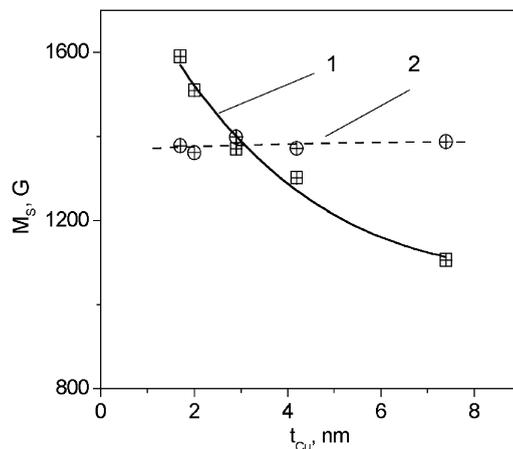
Fig. 6. Magnetization of saturation for buffered (1) and non-buffered (2) multilayers versus the interlayer thickness: 1—Fe(6 nm)[Co(1 nm)/Cu( $t$  nm)]<sub>30</sub>; 2—[Co(1 nm)/Cu( $t$  nm)]<sub>30</sub>. The experimental error is:  $\delta(M) \approx 3\%$ .
