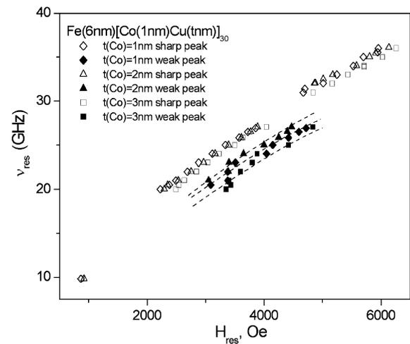
Fig. 2. MLs  $\text{Fe}(6 \text{ nm})[\text{Co}(t \text{ nm})/\text{Cu}(2 \text{ nm})]_8$  ( $t = 1, 2, 3 \text{ nm}$ ). Resonance frequency–field dependence for weak (Co) and sharp (Fe) peaks in “planar geometry”. The experimental error is:  $\delta(\nu) \approx 1\%$ ;  $\delta(H) \approx 1\%$ .
