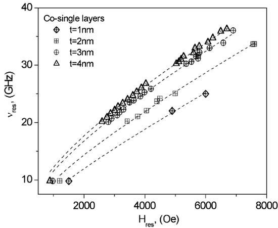
Fig. 3. Single Co-layers. Resonance frequency–field dependence for planar geometry. The experimental error is:  $\delta(\nu) \approx 1\%$ ;  $\delta(H) \approx 1\%$ .
