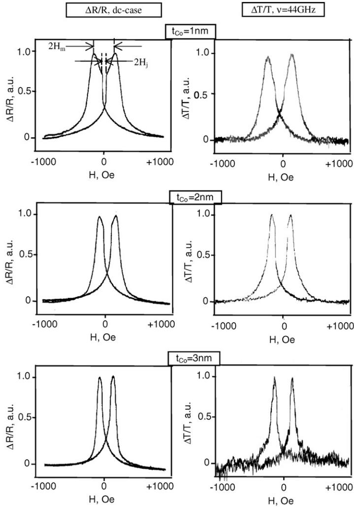
Fig. 7. Magnetoresistance (a) and magnetoimpedance  $\nu = 44$  GHz response (b) for Fe(6 nm)/[Co( $t_{Co}$ )/Cu(2 nm)]<sub>8</sub>.
