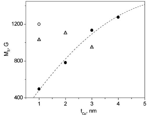
Fig. 4. ESR-technique (dynamic technique). Magnetization of saturation for single Co-layers and for Co/Cu structures versus the Co-layer thickness. The experimental error is:  $\delta(M) \approx 3\text{--}5\%$ . ●—single Co-layers;  $\blacktriangle$ —Co-layers in ML structure Fe(6 nm)/[Co( $t_{Co}$ )/Cu(2 nm)]<sub>8</sub>; ○—Co-layers in ML structure [Co(1 nm)/Cu(2 nm)]<sub>3</sub>.
