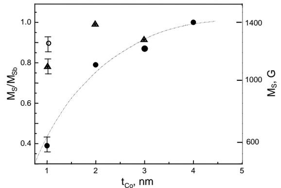
Fig. 5. Vibromagnetometer technique (static technique). Relative magnetization  $M_S/M_{Sb}$  for single Co-layers and for Co/Cu structures versus the Co-layers thickness. ( $M_{Sb}$ —is the magnetization of a reference Co-film by width 30 nm). The experimental error is:  $\delta(M) \approx 10\text{--}15\%$ . ●—single Co-layers;  $\blacktriangle$ —Co-layers in ML structure Fe(6 nm)/[Co( $t_{Co}$ )/Cu(2 nm)]<sub>8</sub>; ○—Co-layers in ML structure [Co(1 nm)/Cu(2 nm)]<sub>3</sub>.
